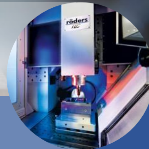
High speed milling of the hardened inserts with up to 42,000 rpm
