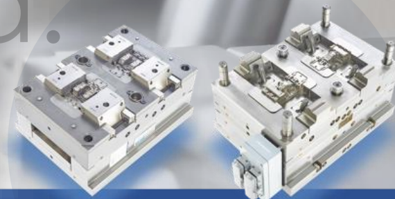
2-cavity injection mold with needle valve hot runner (cascade filling technology) and 4 sliders
