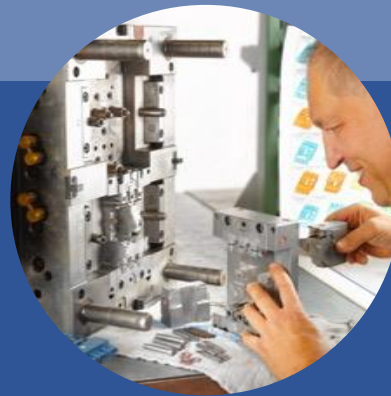
High number of variants due to interchangeable inserts and cores
